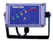
Fitted as a basic and cost effective system, with a transducer fitted integrally into the hydraulics of the truck, the indicator enables simple overloading checks to be performed, often by means of green, amber and red LED indication of load weight. These systems are particularly suitable for applications where the load centre remains constant.
